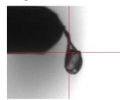
• Ice/frost on the loop/sample or pin:
